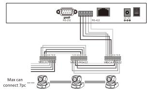
Using RS422 bus connection mode, the third pin Ra of the controller is connected to the TXD IN- of the camera, the fourth pin Rb of the controller is connected to the TXD IN+ of the camera, the first pin Ta of the controller is connected to the RXD IN- of the camera, the second pin Tb of the controller is connected to the RXD IN+
