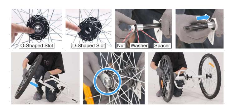
Note: The two rear wheels (13) ARE different and should NOT be mixed up. The wheel with the O-shaped slot goes with the O-shaped hub on the left side of the rear axle while the wheel with the D-shaped slot goes with the D-shaped hub on the right side.
