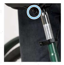
5. To adjust the saddle forward or backward, loosen the two nuts underneath the saddle using the multifunctional wrench, slide the saddle on its support frame until your desired position is reached, and retighten the nuts. Confirm they hold tight and the saddle does not show any wobble.
