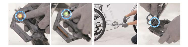
**Note:** The two pedals (8) **ARE** different and should **NOT** be mixed up. The right pedal is marked with an **R** and the left with an **L**.
