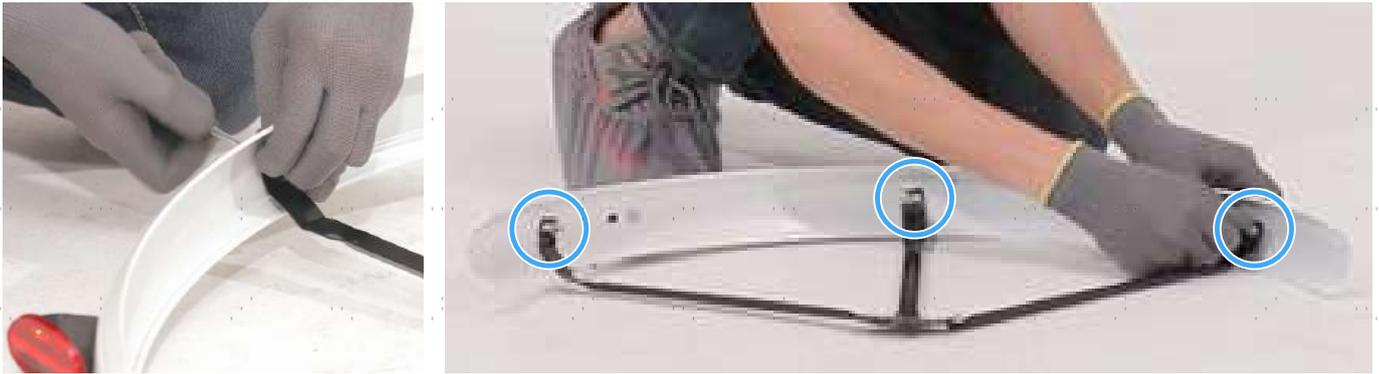
1. Select the appropriate bolts and nuts from the fastener packet, which should match the holes on the rear fenders and the heads of their stays (16).
