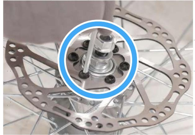
1. Fit the front brake disc (11) onto the left side of the hub on the front wheel (7), aligning their holes.
