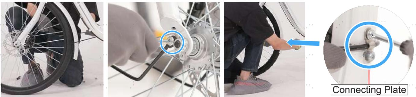
4. Select the appropriate Phillips bolts from the fastener packet, which should match the slots on the front fender stay (12) and the holes beside the front fork's tips. Also find the double-hole connecting plate in the packet.
