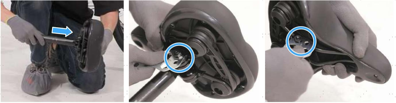
1. Feed the saddle post (6) into the central hole underneath the saddle (5).
