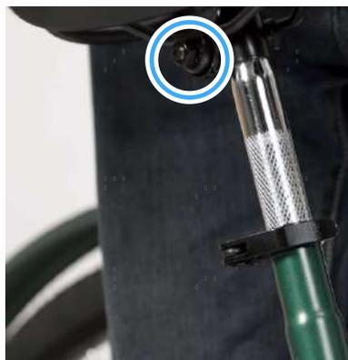
5. To adjust the saddle forward or backward, loosen the two nuts underneath the saddle using the multifunctional wrench, slide the saddle on its support frame until your desired position is reached, and retighten the nuts. Confirm they hold tight and the saddle does not show any wobble.
