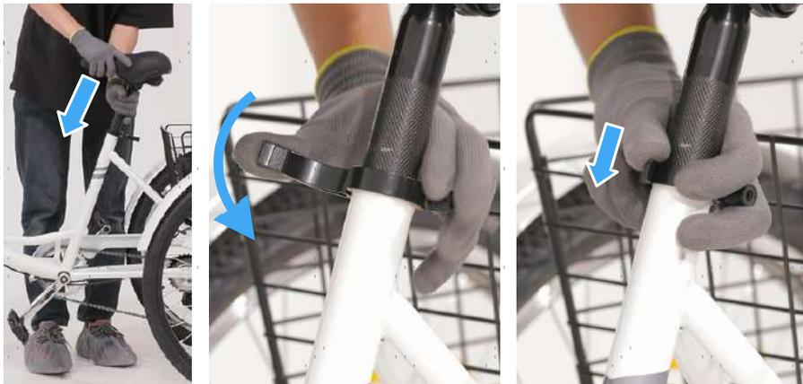
3. Being sure the saddle clamp on the top of the seat tube is open, insert the saddle post into the seat tube until your preferred height is reached.
