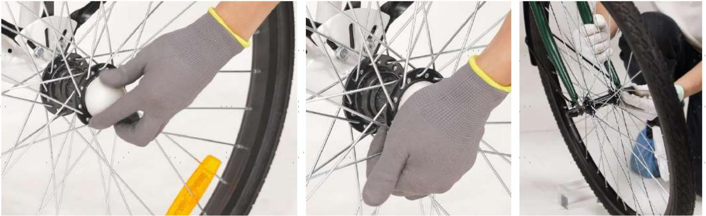
1. Attach the rear wheel caps (26) to the rear wheel hubs, pressing until they are locked in place.
