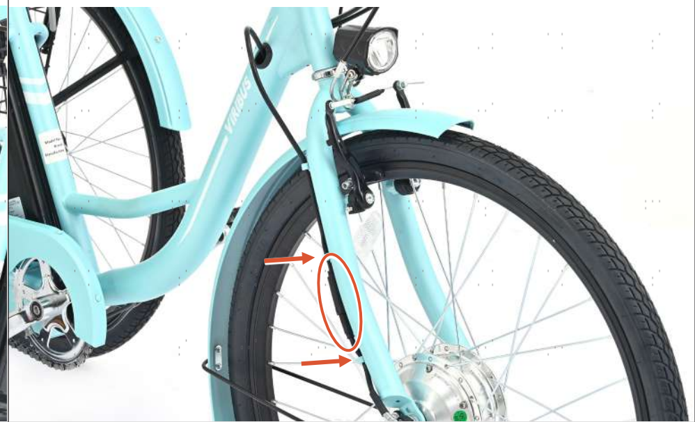
Connect the wiring from the handlebars to the motor. Arrange the wiring neatly throughout the slots along the front fork.
