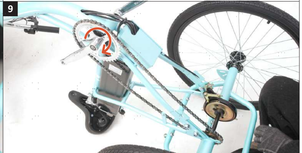
9. Test that the chain moves freely by rotating the right crank arm.
