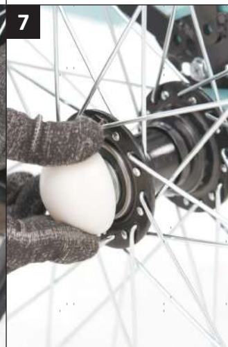
7. Attach the rear wheel caps to the rear wheel hubs, pressing hard until they are locked in place.
