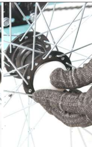
7. Attach the rear wheel caps to the rear wheel hubs, pressing hard until they are locked in place.
