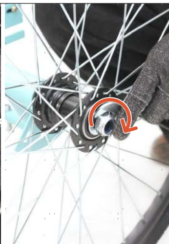
6. Replace the washer and nut, tightening the nut in the same fashion.
