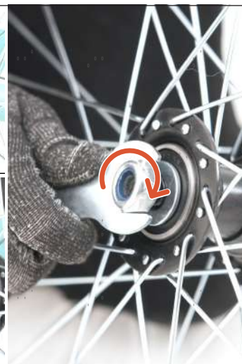
4. Replace the washer and nut, tightening the nut with the 22 mm wrench.
