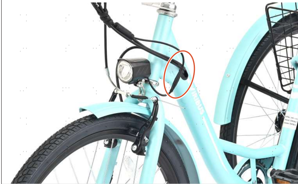
Connect the wiring from the handlebars to the light.
