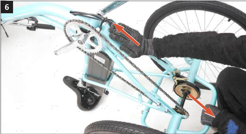
6. Push the main frame forward until the chain is taut.
