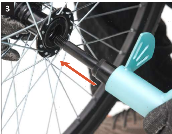
3. Connect the wheel with the D-shaped slot to the hub.
