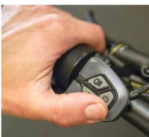
**3. Power Off Battery**Hold battery button for 3 seconds.
