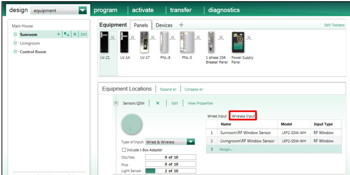
Figure 9: Assign Radio Window Sensors to a QSM Wireless Input
