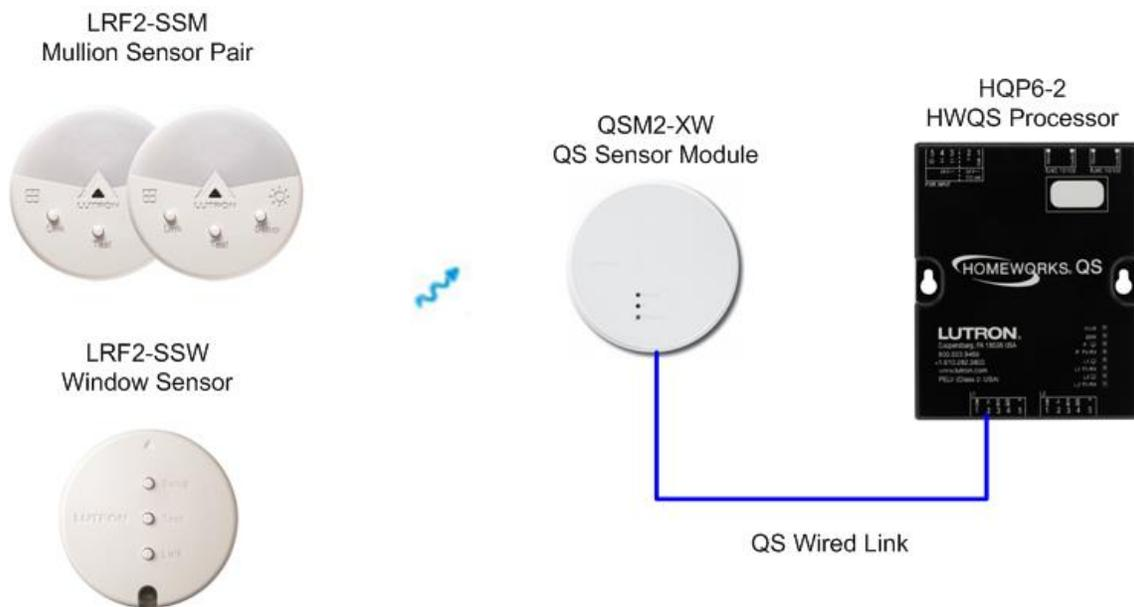
Figure 1: Radio Window Sensors Communicate with the QSM
