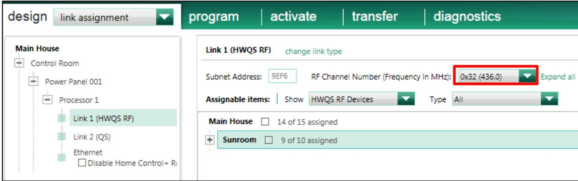
Figure 20: Configuring the RF channel of a HomeWorks QS RF link
