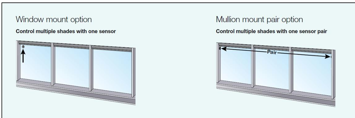
Figure 3: Window Sensor Mounting Options
