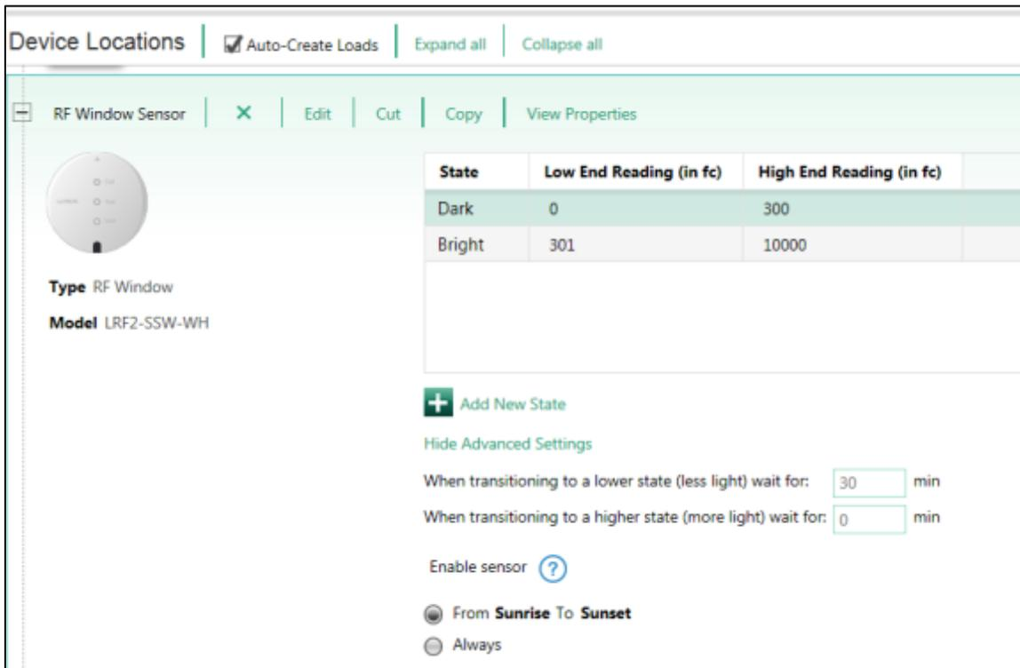
Figure 5: Adding a Radio Window Sensor to the Project
