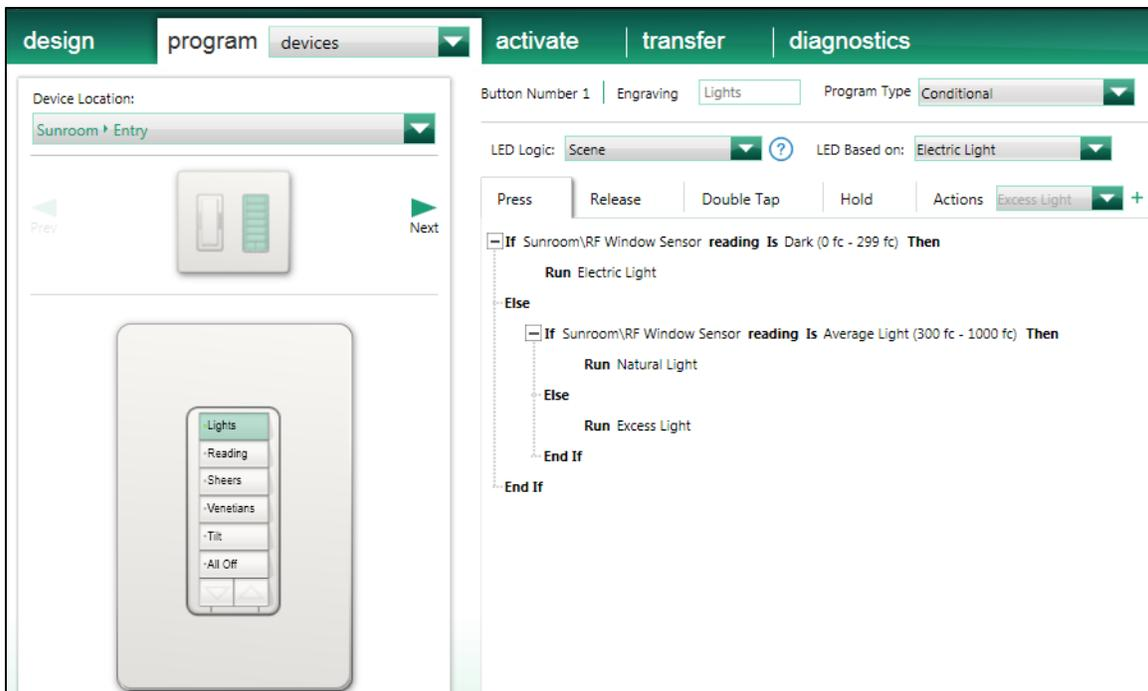
Figure 15: Keypad Button Programming
