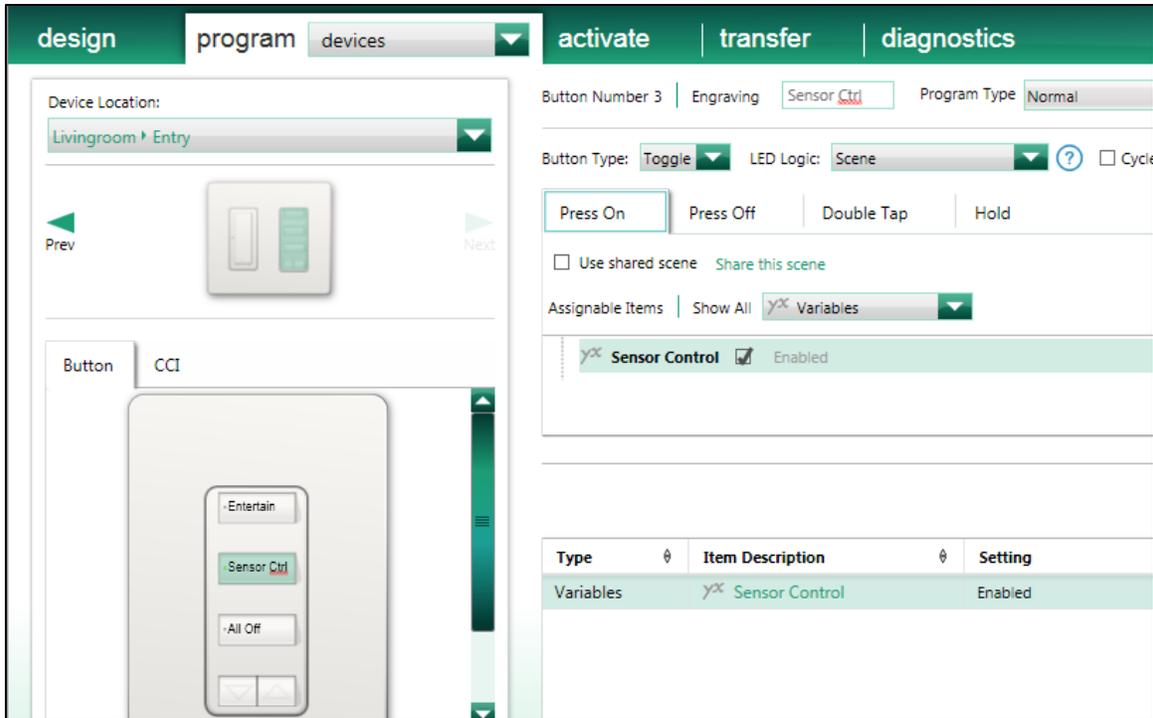
Figure 12: Variable to Control Window Sensor Programming
