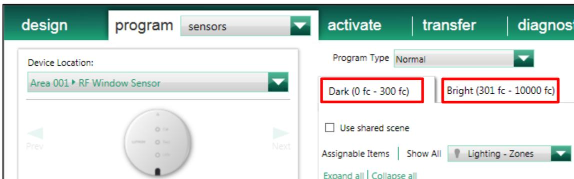
Figure 6: Programming Tab for Window Sensors
