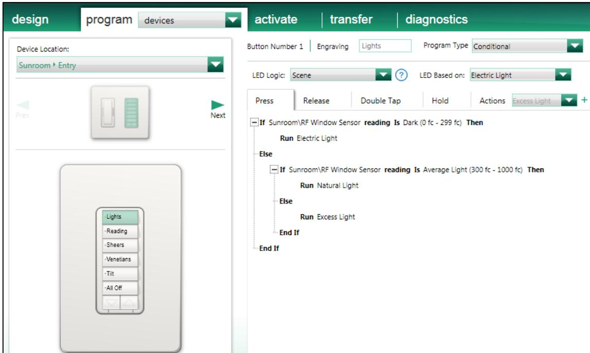
Figure 15: Keypad Button Programming
