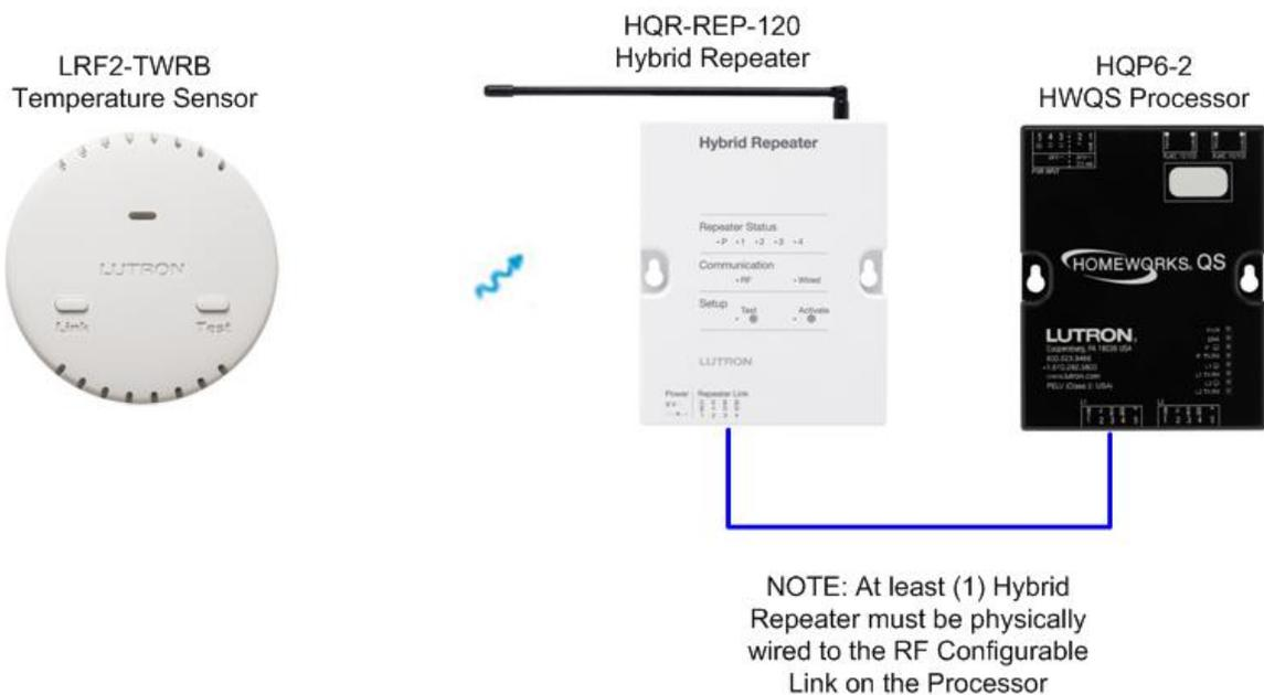
Figure 2: Temperature Sensors Communicate with the Hybrid Repeater
