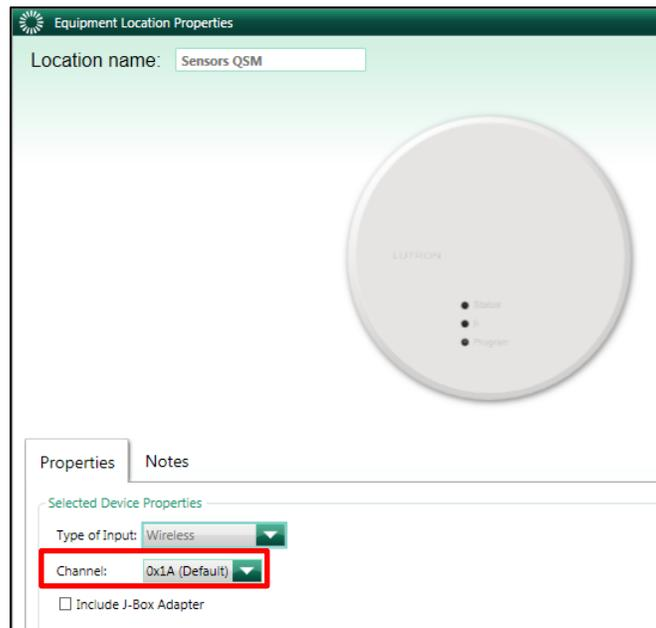
Figure 19: Selecting the RF Channel of a QSM
