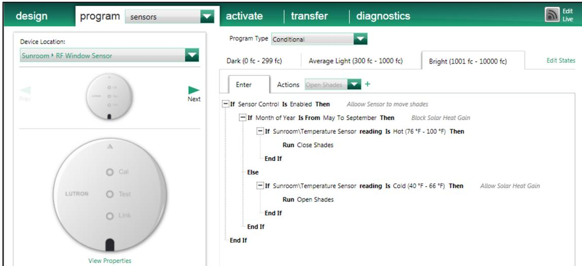
Figure 14: Radio Window Sensor Programming with Temperature Input
