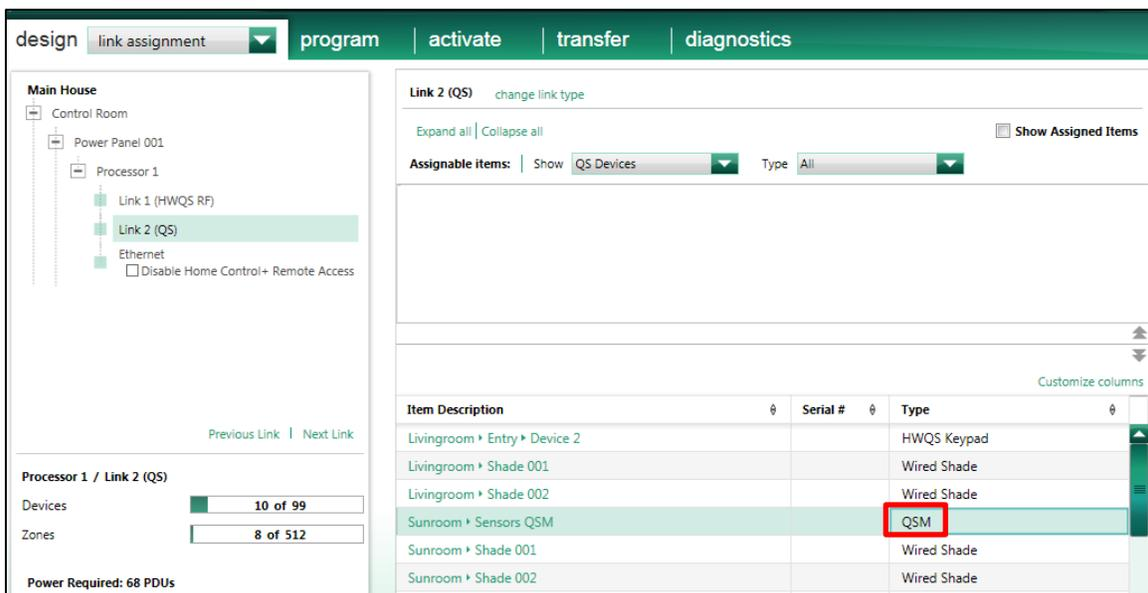
Figure 10: Link Assignment for QSM
