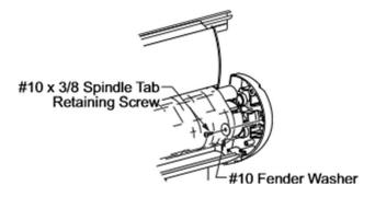
Step 4: Remove the end cap on one side. (the side you will be pulling the fabric out of) These will be the remaining 2 screws left in the end cap.
