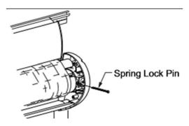
Step 3: Pull the screw that secures the hardware inside the end cap on both sides.
