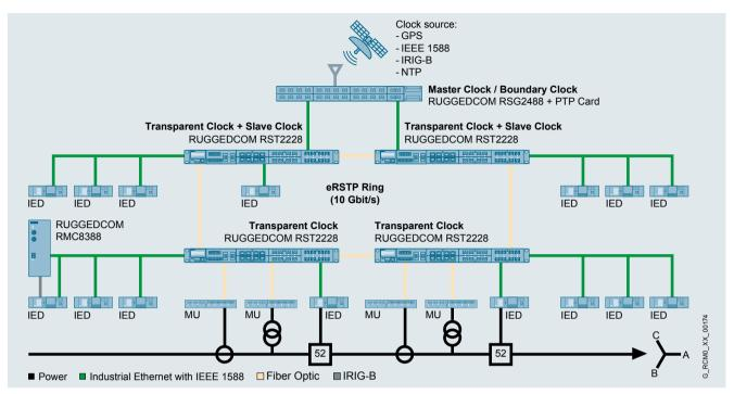
Up to 24 modern IEDs or other IEEE 1588 slaves can be connected directly to the RUGGEDCOM RST2228 via Fast Ethernet or via Gigabit/s ports.
