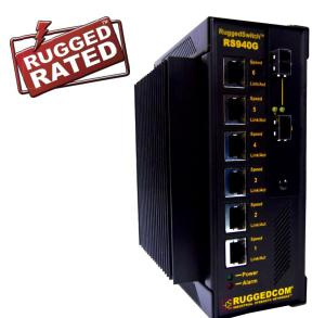
The RuggedSwitch® RS940G is an industrially hardened, fully managed Ethernet switch providing six or eight ports of Gigabit Ethernet. Six 10/100/1000BaseTX triple speed copper ports are standard. An additional two gigabit fiber or copper ports can be added. The RS940G provides a cost effective way of connecting a cluster of field devices to a Gigabit Ethernet backbone.
