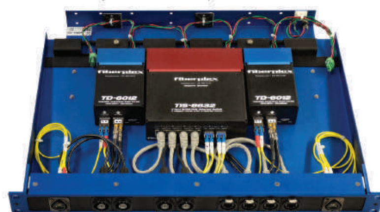
Preconfigured 4 HD-SDI Video plus 10/100/1000 Ethernet
