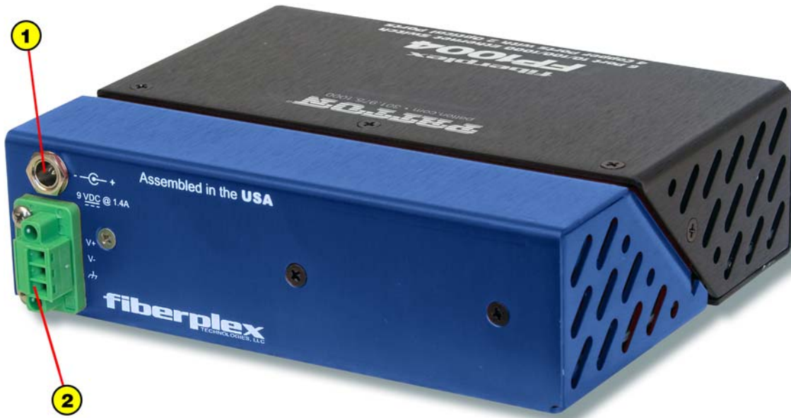
Figure 9. FP1004E rear panel ports
