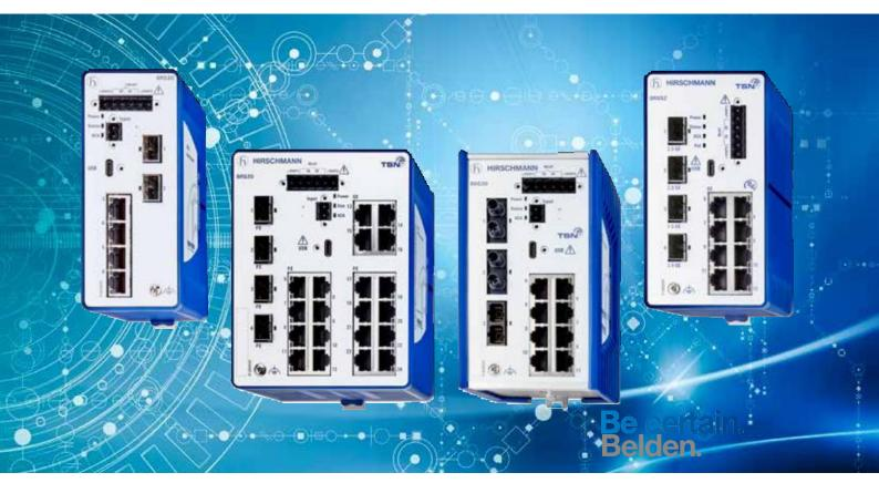
The Hirschmann BOBCAT Switches offer enhanced flexibility and interoperability for simple maintenance and future-proof operation due to tri-speed SFP ports and downwards compatibility for existing infrastructure.
