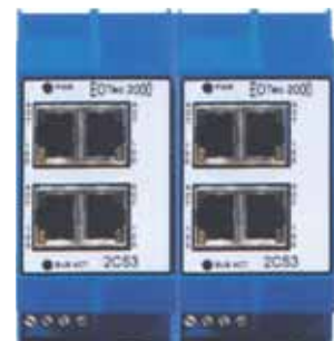
Two 2C53 Ethernet Switches
