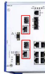
RSPL30 08 02 207 YT 2x Combo ports (GE/FE) 2x FE SFP-slots 6x FE TP, RJ45
