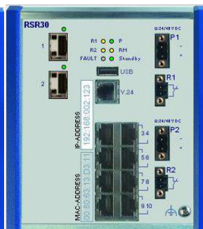
RSR30 08 02 06 06 T1 2x SFP slot (GE) 8x 10/100BASE-TX(RJ45)
