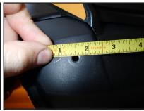
4. Now slide the hood forward enough that you can work behind the nose of the hood. Measure from the bend in the hood and make a mark at  $2\frac{1}{4}$ ". Measure down from the top of the hood 7/8" and make a
