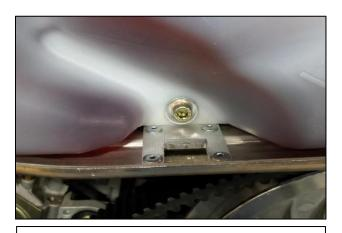
4. Install the previously removed flat washer onto the new bolt and install into the new bracket, holding the oil tank in place.
