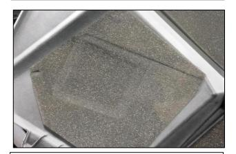
8. With the motor assembly in place, install the side panel. Now is a good time to remove the sticker from the side panel while waiting for imprint to appear on the side panel foam.
