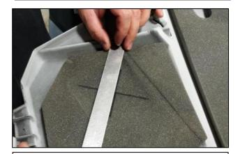
9. Using a straight edge, draw a line from corner to corner within the imprint as shown.
