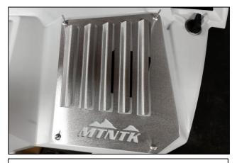
11. Install the vent plate to match body lines of the panel. Mark first, then drill and install the four aluminum expanding rivets as shown.
