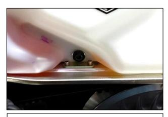
1. Start by removing the left hand side panel. Remove the oil tank retaining bolt. Save the flat washer and discard the bolt.
