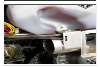
7. Mount the Blow Hole and route the wires as shown so there is no slack above the primary clutch. Plug into the factory DC power port.
