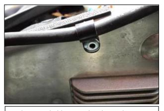
6. Place wire holder onto the Blow Hole wire then rivet into place as shown.
