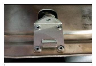
3. Place new bracket provided in the stock location. Place two steel rivets into the stock holes, then mark where to drill remaining two. Drill into the aluminum shelf and install rivets
