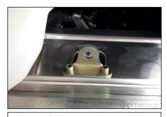
2. Using a 3/16" drill bit, carefully remove the rivets and bracket and discard both.
