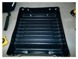
5. Install one  $1/4 \times 5/8$ " button head screw per hole with a 1/4" flat washer and Nylon lock nut on the inside of the tray. You may have to use a longer screw to crush the plastic before installing the 5/8 bolt, flat washer and nut. The goal here is not to have any threads exposed that could wear the material.
