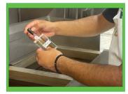
Using a test kit to look at color could be the difference between "the same oil life" and saving thousands per fryer!
