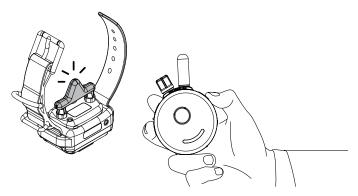
If you need to check your unit, hold the test light against the contact points on the collar receiver. This test will let you know that the collar receiver is generating the proper sensation to the dog, it should brighten in a smooth fashion as the dial is turned up.
