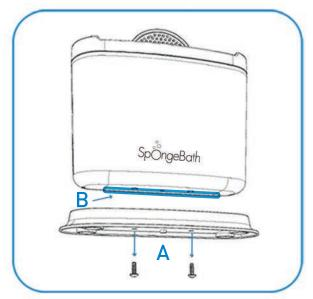
(A) Unscrew two Countertop Stand screws and remove Countertop Stand to (B) Reveal Slot on bottom of Tub.
