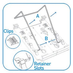
4 • To adjust height for an overmount or undermount sink – (A) Unlatch steel Hanger Bar by pulling it out of Clips. (B) Squeeze lower part of Hanger Bar together to slide out of Retainer Slots, re-insert into desired slot height, and snap Hanger Bar into clips.
