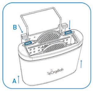
2. (A) Align the bottom hook on Mounting Bracket with Slot on bottom of Tub and insert. (B) Snap top Support Arms on Mounting Bracket into the indents on Cap.
