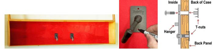
**Step 3**: From the back of the case, insert the T-Nuts with the prongs-side facing into the 2 holes as shown in the 1<sup>st</sup> photo below. Push the T-nut into the back panel as much as you can.
