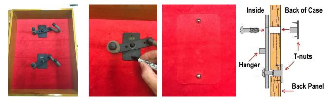
Step 3: From the back of the case, insert the T-Nuts with the prongs-side facing into the 2 holes as shown in the 1st photo below. Push the T-nut into the back panel as much as you can.
