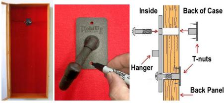
**Step 4:** Position the hanger plate from the inside to align with the 2 holes/T-nuts. Use the 2 black screws to attach hanger as shown in 2<sup>nd</sup> photo. You will need to screw very tightly, as this will force the T-nut prongs to press into the back panel. A power screwdriver is best for this. The attached hanger should look like the 2<sup>nd</sup> photo from
