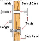
**Step 3**: From the back of the case, insert the T-Nuts with the prongs-side facing into the 2 holes as shown in the 1<sup>st</sup> photo below. Push the T-nut into the back panel as much as you can.
