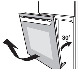
3. Open the door rotation bracket assembly. Refer the action in the following picture.
