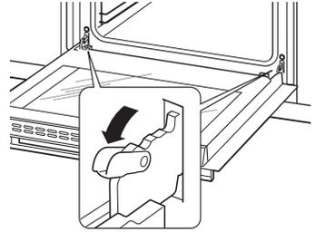
2. Close the door to an angle approximately 30°. Hold the door with one hand on each side. Lift up and slowly pull the door out from the oven.
