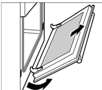
3. Close the appliance door until you feel resistance at an angle of around 15° (in relation to the closed appliance door).
