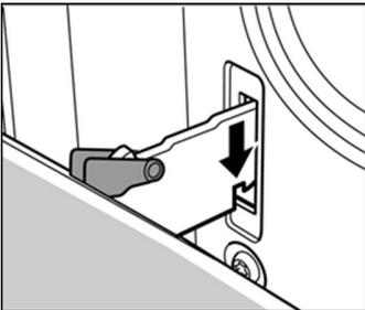
3. Position the door so that the hinge grooves engage on both sides.
