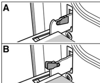
The hinges of the appliance door are each secured by a locking lever. When the locking lever is folded in (A), the appliance door is secured. It cannot be unhinged.
