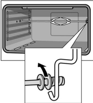
2. Carefully withdraw the rotary spit from the recessed adapter in the side panel and remove it from the oven.
