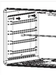
2. Take hold of the top of the hook-in rack and screw on the screw on the bottom the hook-in rack again.
