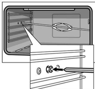
2. If the oven has been preheated, only attach the rotary spit if you are using an oven cloth or wearing (thermal) oven gloves. To attach the spit, slide one end into the recessed adapter in the left-hand side panel of the cooking compartment.
