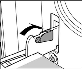
5. Fold in the locking levers on both sides.
