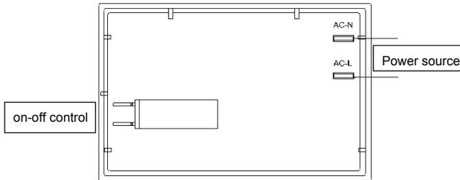
As shown in the picture, on-off control is used to control heating components of oven, the left is power source which can be connected under the 220V.
