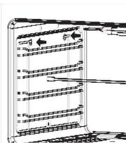
2. Pull the hook-in rack slightly downwards and insert the lower hooks into the drill holes.
