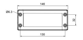
The DES 24 cable entry system consists of a splittable frame designed to accommodate small (SPP), multiple (X) or large (SPG) grommets for cables with and without connectors. The grommets can be freely positioned into the frame.
