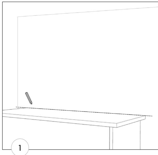
1. Determine the placement of the most lower slatwall profile section and then, using a level, mark a line across the entire length of the surface to be covered.
