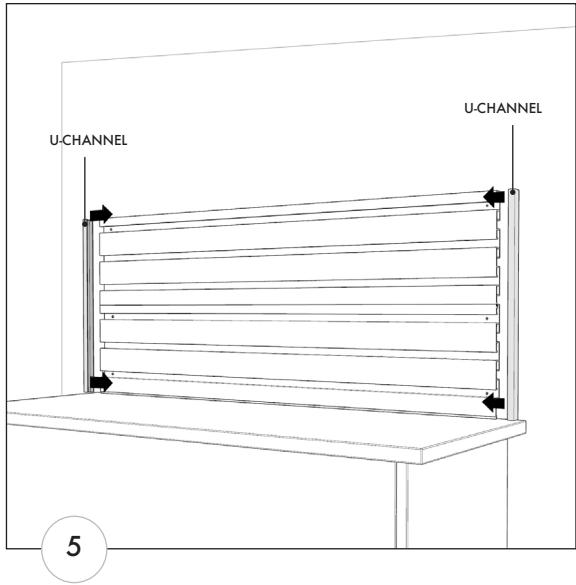
5. Use the provided u-channel to hide the edge of the slats and provide a properly finished look. Slide the u-channel along one side of the slats, **fully tightening the screws on that side to pinch it in place**. Repeat the procedure for the opposite u-channel.
