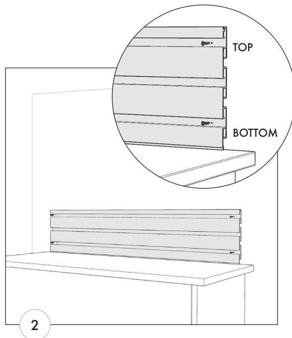
2. Place the first 6" slatwall piece onto the surface with the bottom aligned with the level line.
