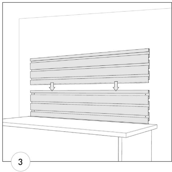
3. Place the next slatwall profile section onto the profile from step 2). Check level.
