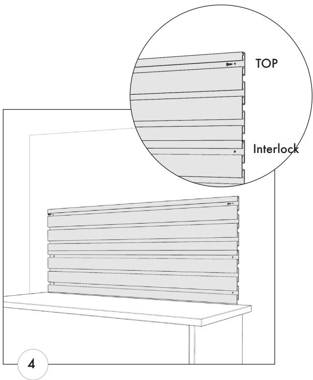
4. For additionnal slatwall panels, screw on top only.
