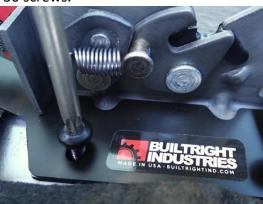
6. Closing the rear seat back will always require a firm push, but when closing the rear seat back for the first time, you may need to realign the 'catch bar' on the back of the cab. When we lifted the bottom of the seat, the 'catch bar' moves up. Some experimentation and you'll have it no problem.
