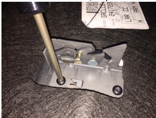
3. Prepare the BuiltRight seat release bracket by slipping the strap through the strap retainer as shown below.
