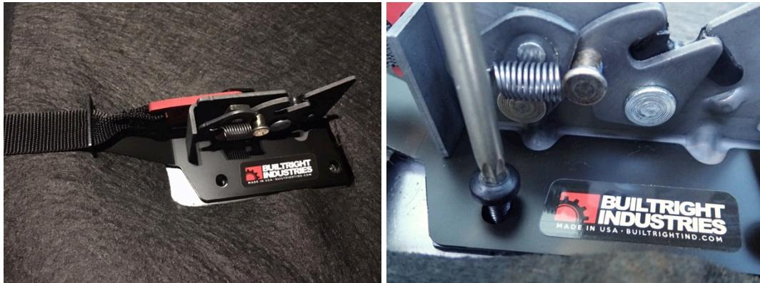
6. Closing the rear seat back will always require a firm push, but when closing the rear seat back for the first time, you may need to realign the 'catch bar' on the back of the cab. When we lifted the bottom of the seat, the 'catch bar' moves up. Some experimentation and you'll have it no problem.
