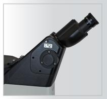
Standard side-mount camera port allows easy access to camera controls.
