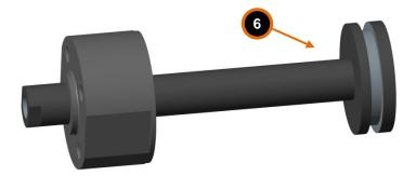
Insert the piston with the cover back to the actuator and screw the cover back in place. When both ends are fully tightened, centers of the pneumatic fittings must be horizontally aligned. Be careful about the sealing when removing or assembling the actuator. Check lubrication when assembling the actuator (see servicing below).
