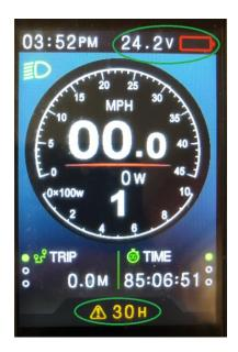
6. Press and hold the " + " and " – " buttons at the same time to reset the counter in the lower right corner of the display. This will allow you to monitor how long the display has been charging
