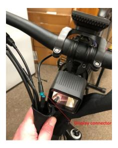
2. Plug charger into the connector of the APT850C display. Be sure to align the indexing features.
