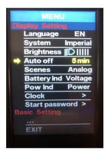
8. Use the power button to select "Auto off" and use the " + " button to change the setting to OFF
