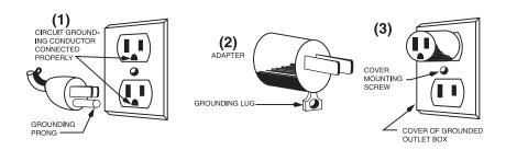
If a grounding-type outlet is not available, an adapter, shown in Figure 2, may be obtained so that a 2-slot wall outlet can be used with a 3-prong plug. As shown in Figure 3, the adapter must be grounded by attaching its grounding lug under the screw of the outlet cover plate.
