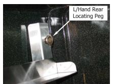
b. Locate the top front of the rack over the locating peg at the top front LH side of the oven.
