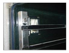
b. Remove the 4 screws securing Support Frame, Gasket and Glass Lens to the light fitting and carefully remove items, taking care as glass lens is a loose fit in the support frame.
