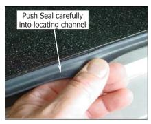
f. Press the door seal into the locating groove in the front face of the oven until the seal is properly located all around the oven.
