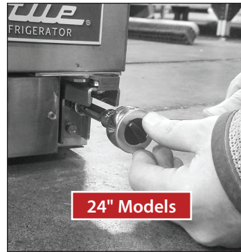
Fig. 1. The 24 and 27 models use different lower hinges.
