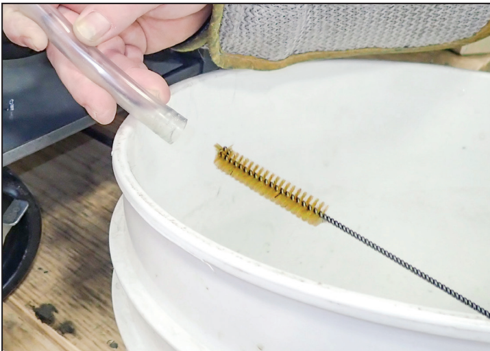
Fig. 2. Catch trapped liquid in a large container.
