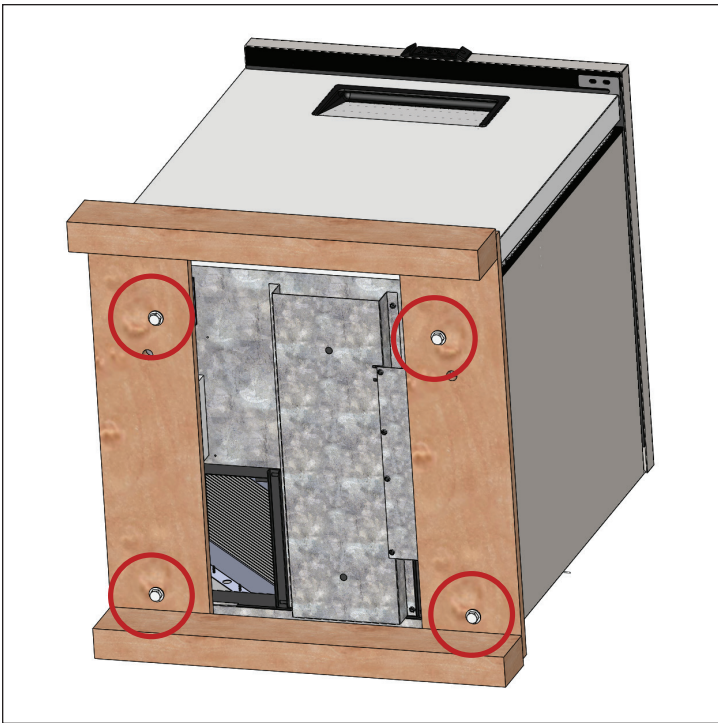
Fig. 3. Remove all shipping bolts.
