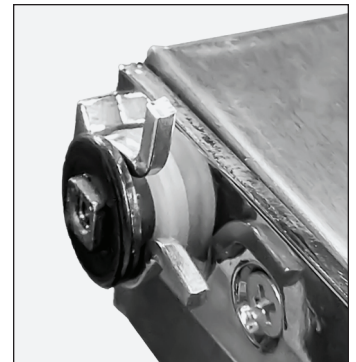
Fig. 7. Keep the washers in their original order.
