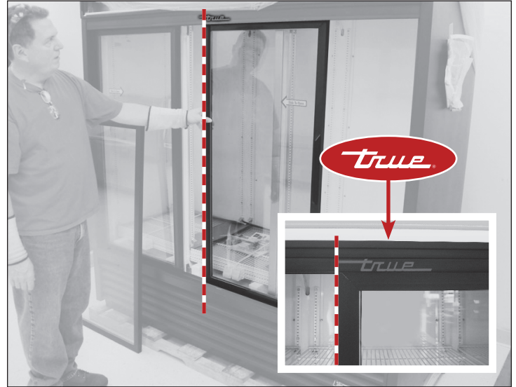
Fig. 5. Align the right door's left edge with the TRUE logo's left edge.
