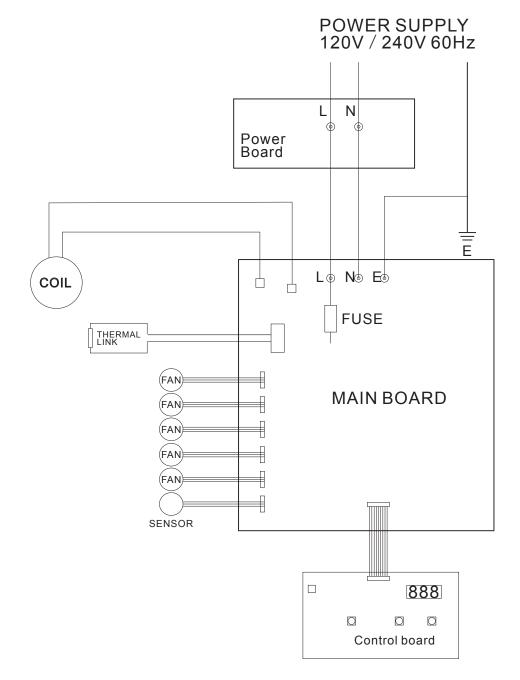
This circuit diagram has been provided to assist qualified electricians; only SPECTRUM<sup>™</sup> service agents or qualified electricians should carry out repairs if required.
