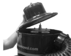
Thoroughly clean all parts, and block of the machine with cold water and detergent.
