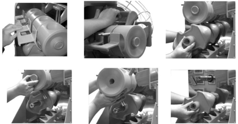
Remove the squeezer drum by unscrewing the screw. Remove the second squeezer male part.
