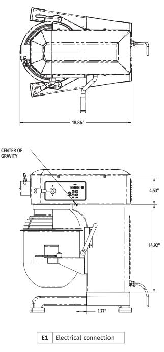
MACHINE ELECTRICAL SPECS: 120/60/1 – ETL Listed
