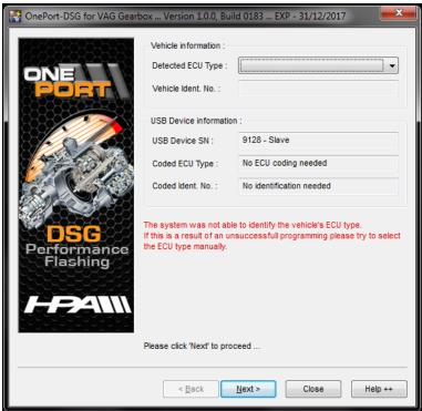
35) Select the corresponding DSG Gearbox type from the pull-down bar at the top of the screen beside "Detected ECU Type" the same as you selected during the read process.
