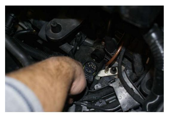
17) Now install the adapter cable's round connector onto the DSG mechatronic. Rotate the tap clockwise to click it in place.
