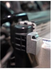
**Step 29**Bring the top of the radiator forward and clip together on both sides of the intercooler.
