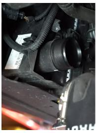
Step 5 Disconnect the charge pipes from underneath the car.
