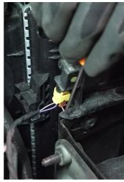
**Step 20**Unclip the airbag crash sensors (yellow)
