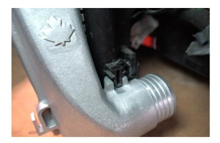
**Step 28**Seat the OE radiator into the slot on the HPA Intercooler.
