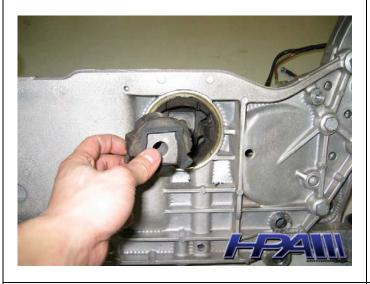
6. Use dish soap to lubricate core interlock mount and install in to sub frame making sure the recess in the mount matches up with the corresponding existing pendulum rod
