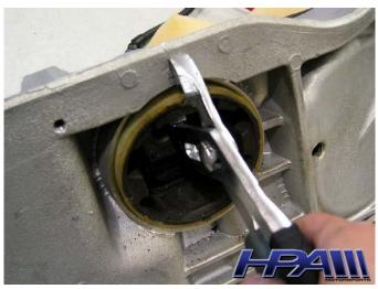
6. Secure core interlock mount with OE bolt. Torque to 50nm plus an additional 1/4 turn
