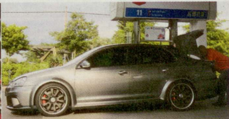
Refuelling not so straightforward. To make space for the rear axle, the car now keeps the fuel cell in the trunk. Better not keep the groceries in there!
