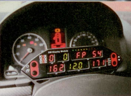
(left) Stack display on steering column provides everything you need to know. Just as well 'cos the speedo and fuel gauge were not working!
