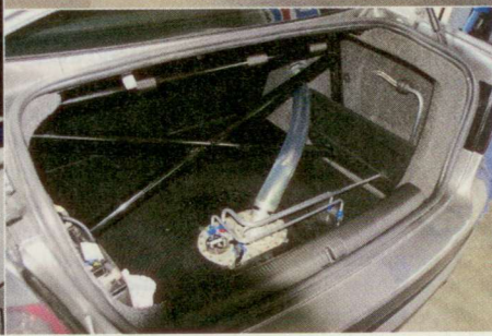
Refuelling not so straightforward. To make space for the rear axle, the car now keeps the fuel cell in the trunk. Better not keep the groceries in there!
