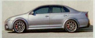
Jetta R GT crouches on huge 9.5x19 custom-built forged aluminum modular Avus wheels with DTM-style center locks, wrapped by 265/30-19 Michelin Pilot Sport 2 ultra-performance radials-and that's just in street trim. When the Jetta arrives at the track, the integrated AP Racing air jacks can be deployed to quickly mount race wheels and rubber: 9.5x19-inch. Avus DTM-spec center lockers and 265/30-18
