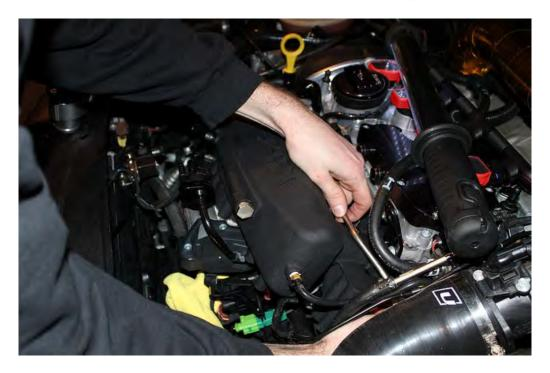
30) Reconnect Previously Removed Fuel Lines, PCV Lines, Vacuum Lines, Breather Lines:
