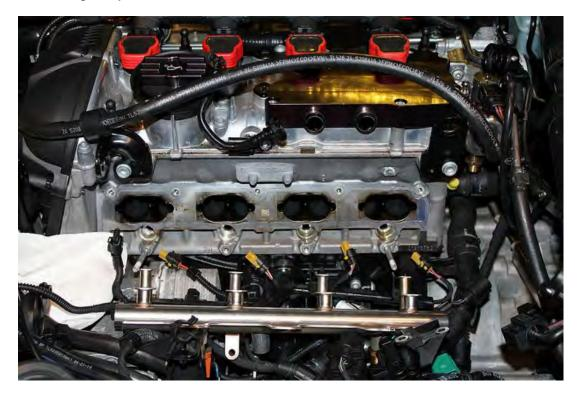
NOTE: Carbon Buildup (5,000 miles on new engine):
