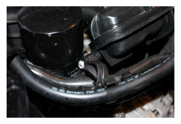
20) Remove Oil Filter (allows for easier access for the remainder of the installation):
