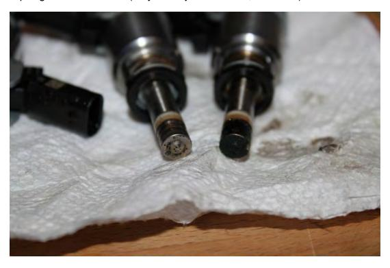
24) Replace Fuel Injector O-Rings with OEM Fuel Injector Service Kit:
