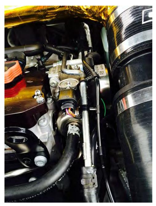
**NOTE:** It would be a good idea to double check the PCV valve on top of the valve cover. These are known to fail, especially on higher boost applications. Copy the part number on the top and ask your local dealer for the latest iteration of it.
