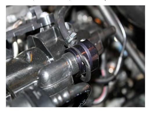
5) Remove Connectors On Valve Cover:
