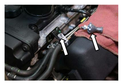
39) Trim notch in engine cover to provide clearance for oil dipstick and install engine cover. Add 2 inches of wire to intake air temperature sensor wiring with supplied butt connectors. After crimping connectors, please heat with heat gun or lighter to seal connections.
