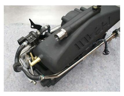
27) Install provided flapper motor stopper and flapper motor with supplied and M6 bolts according to the following pictures.
