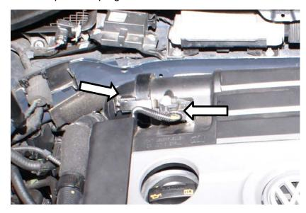
b. Remove duct from radiator support
