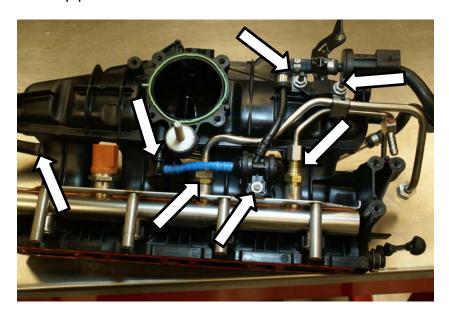
24) Make sure all connections are loosened and ensure the fuel rail is free from intake manifold, connectors, and lines. Remove fuel rail from intake manifold.
