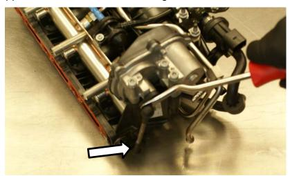
26) Re-fit parts to HPA Intake Manifold with supplied bolts and washers and torque to 10 Nm. Fuel rail is no longer bolted directly to the intake manifold. Please be patient in fitting the fuel rail to the manifold as tolerances may be tight.
