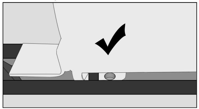
5. ON THE INSIDE ON THE LEG, PLACE THE L-BRACKET INTO THE REAR SLOT, MAKE SURE THE HOLE ON THE L-BRACKET AND REAR HOLE OF THE LEG ALIGN, THEN INSTALL BOLT BY HAND FIRST THEN TORQUE TO 26 FT-LBS.
