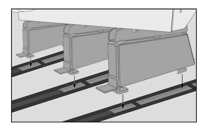
4. PUSH THE SEAT FORWARD TO ENSURE LEGS ARE FULLY INSET AND FULLY PUSHED FORWARD INTO THE FLOOR RECEIVERS.
