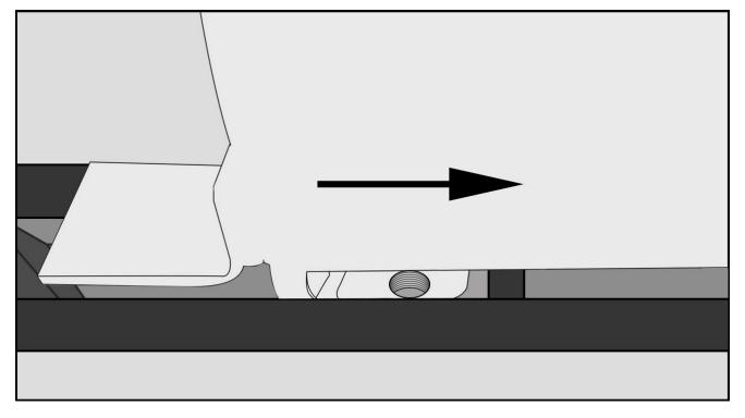
ONCE LEGS ARE FULLY INSET AND FULLY PUSHED FORWARD INTO THE FLOOR RECEIVERS, YOU ARE READY TO PROCEED TO NEXT STEP.
