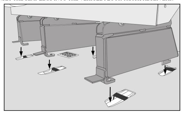
5. PUSH THE SEAT FORWARD TO ENSURE LEGS ARE FULLY INSET AND FULLY PUSHED FORWARD INTO THE FLOOR RECEIVERS.
