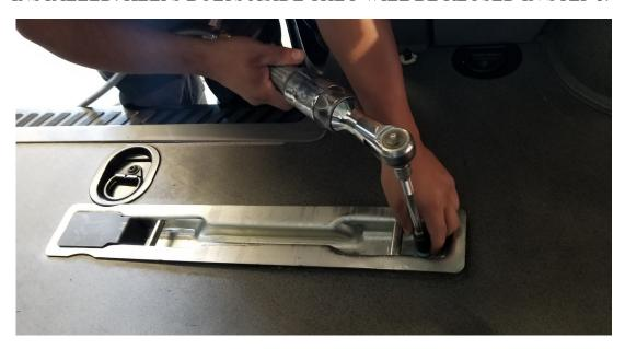
REMOVE FRONT PLASTIC GUARDS FROM OEM FLOOR TRACKS.
