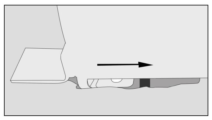
ONCE LEGS ARE FULLY INSET AND FULLY PUSHED FORWARD INTO THE FLOOR RECEIVERS, YOU ARE READY TO PROCEED TO NEXT STEP.
