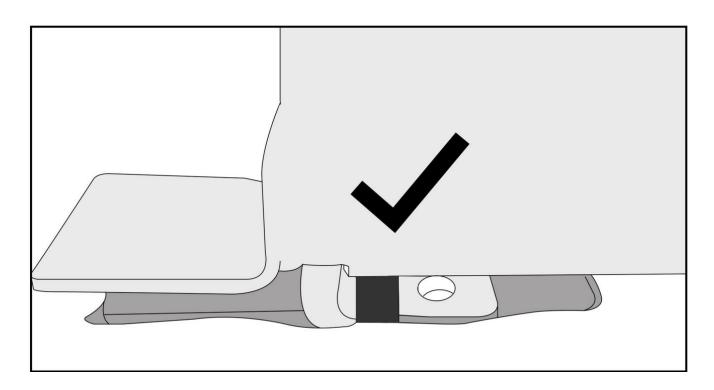
6. USING THE OEM BOLT THAT WAS REMOVED EARLIER IN STEP 2, PLACE BOLT THROUGH L-BRACKET AND SECURE DOWN TO OEM TRACK BY HAND.
