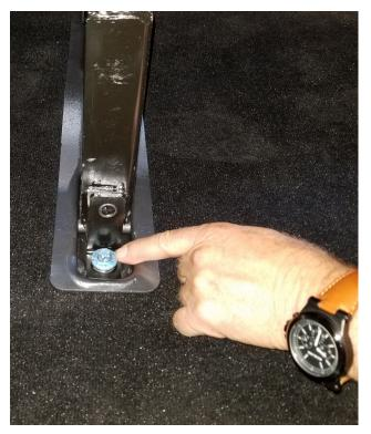
7. ALIGN L-BRACKET TO BACK OF LEG AND FASTEN BOLT, L-BRACKET AND NUT TO REAR OF LEG BY HAND FIRST.
