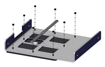
8 | Using 7 x WN20 nuts, secure BKT03 and SK03 to TPB03 by tightening from the underside. Whilst doing so, secure the LED strip (with Inovus logo facing downwards) at the position shown in the image
