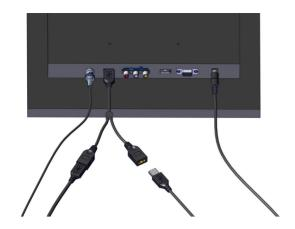
33 | Finally, connect the Micro USB cable to the remaining USB port on the USB splitter.
