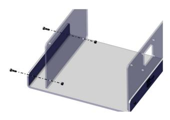
3 | Repeat Step 2 for the rear panel U01, using a further 2 x M5B8 bolts and 2 x WN20 nuts.
