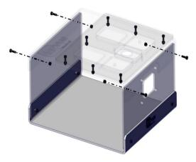
9 | Place TPB03 over the upright panels. Aligning the bolt holes, secure it in place using 4 x M5B8 bolts and 4 x WN2 nuts.
