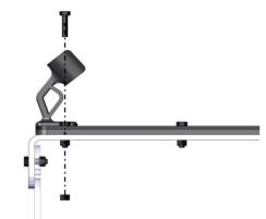
10 | You may now take the scope bracket (INOPPMBKT). Align the bolt hole on the base of the bracket with the front (middle) bolt hole of BKT03. Secure the bracket in place using 1 x M5B12 bolt and 1 x WN20 nut.
