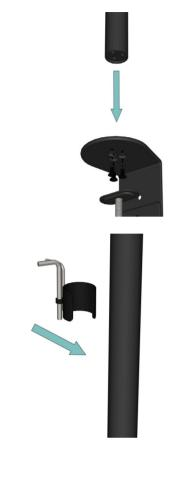
17 | Using the three black bolts provided, attach the black post to the C-clamp.
