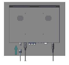
28 Connect the female end of the BNC extender to connector at the back of the monitor.
