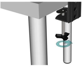
22 | With the bracket fully assembled, anchor it to your chosen work surface by turning the handle until it is tight.
