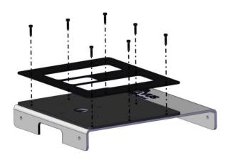
7 | Take the BKT03 bracket and place it over the SK03 skin. With the bolt holes aligned, place 7 x M5B12 bolts into position as shown. At this stage, leave the front (middle) bolt hole free.
