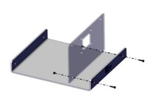
2 | Using 2 x M5B8 bolts and 2 x WN20 nuts, screw the UHDM front panel into position as shown.
