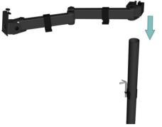
19 | The swivel arm should be preassembled Slide this onto the black post.
